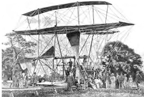
Hiram Maxim at the controls of a famous but impractical invention—his steam-powered, rail-mounted biplane made of tubular steel and canvas biplane in 1894. It 'flew' for about 200 metres during a trial in 1895 but then broke an axle and was so seriously damaged that Maxim abandoned the project.
