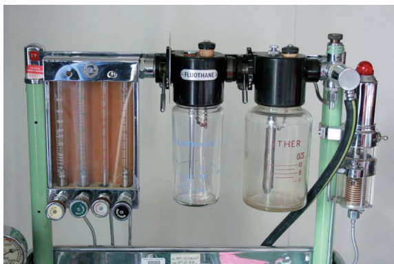
The back bar of a 1950's Boyle's machine — the CO 2 rotameter is second from the left.
