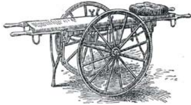
The 'new St John' litter fitted with 'Regulation Military Stretcher'. It has central 'Y-shaped' retractable legs fore and aft.
