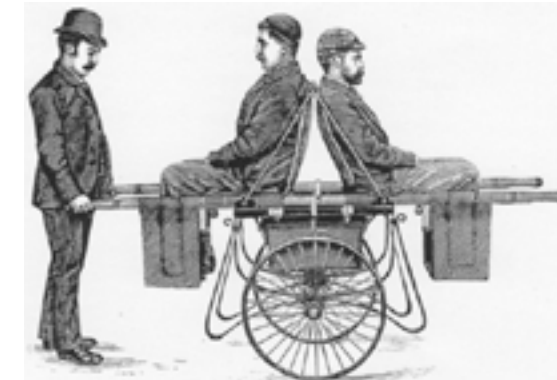
The extraordinary ‘Furley-Headley’ litter. It could carry two patients sitting (left) or one lying (right), and the legs could be raised and lowered. How stable it was when carrying two patients is a matter that invites speculation.
